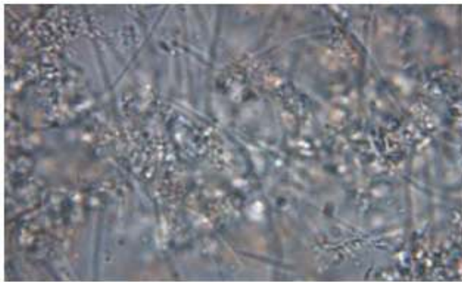
Figure 1 Stirling WWTP mixed liquor, phase contrast microscopy, 1000X magnification
