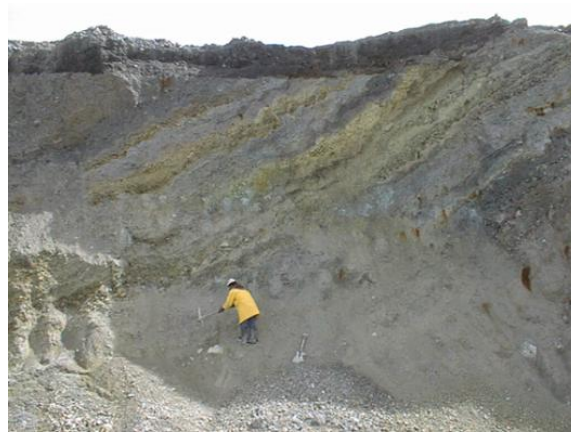
Figure 4. Autopsy of a waste dump constructed by end-tipping. Note the pathways for oxygen ingress (coarse material). Figure courtesy of Environmental Geochemistry International Pty
