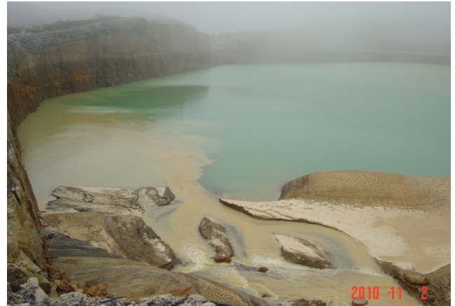
Figure 20. Influent via the Mangatini Stream into the Mangatini Sump. Note limestone dosing turbidity
