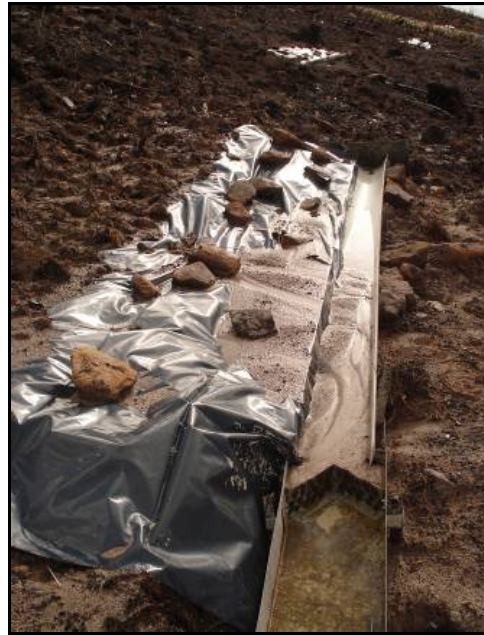
Figure 10. Erosion control gutter used to measure sediment loss from trial plots. Further details of the design, methodology, and results are available (Shadbolt and Weber, 2007).
