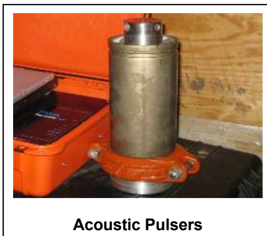
Figure 9. Acoustic Pulsers used for Pipe Wall Assessment (PWA)
