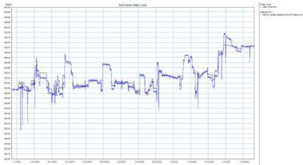
Figure 2-6 Comparison between measured and simulated water levels at Valetta Head Pond. The measured values are shown in blue
