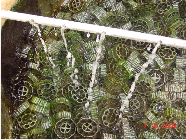
View of top surface of Plastic Media in Pilot Biological Trickling Filter showing screened wastewater distribution onto the Media, December 2005
