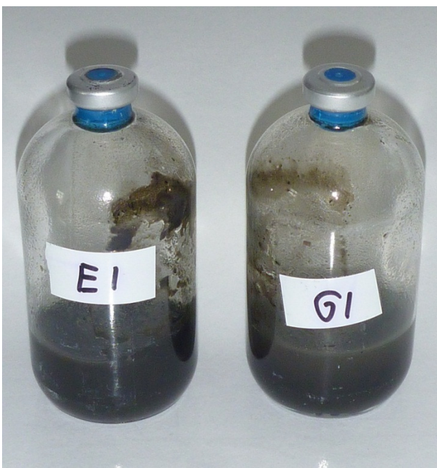
Photograph 1: Two 160 ml serum bottles with butyl rubber septum as used in BMP tests
