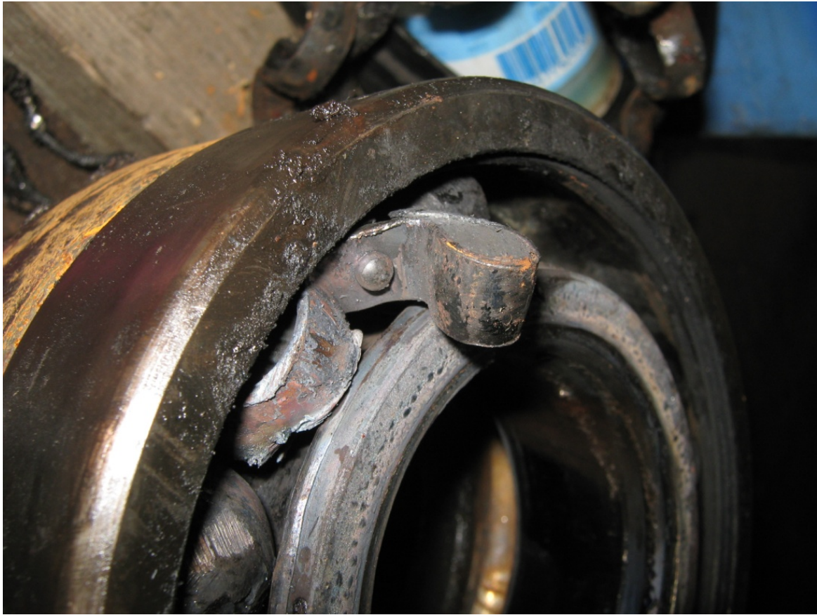
Photograph 13: Bearing from Pump2 showing typical damage.
