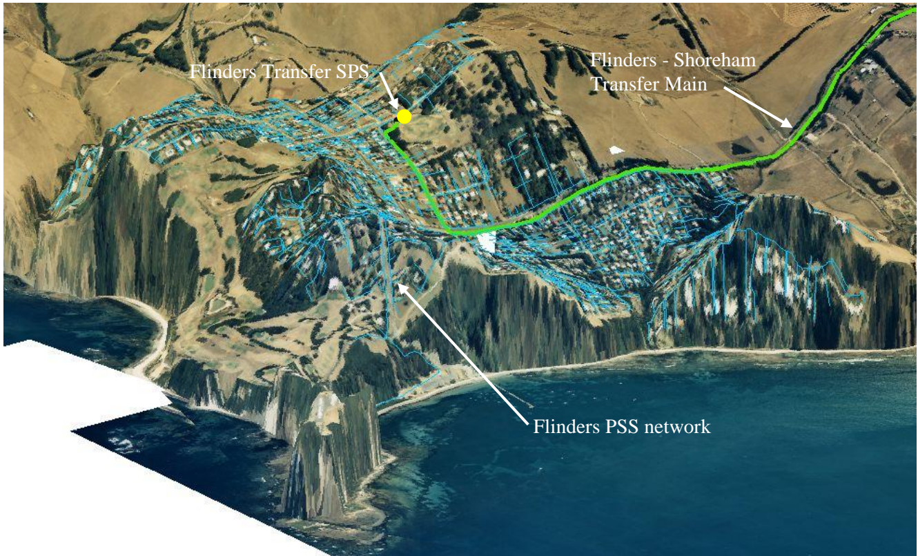
Figure 7: Flinders Pressure Sewerage network – Aerial Photo
