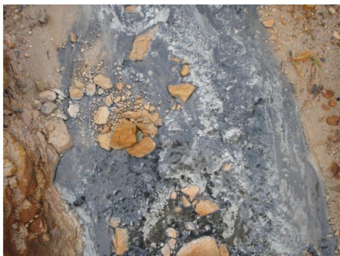
**Photograph 1. Black precipitate at the effluent discharge point** for the Manchester Street seep mussel shell bioreactor at Stockton coal mine.
