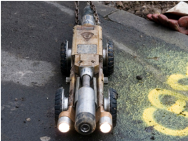
Photograph 1: "CCTV camera used to inspect pipes with no or minimal flow"
