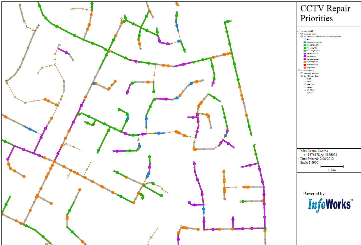
Figure 7: InfoNet plot of assessments in WW network based on CCTV, PDAT, Pipe Profile and MH Level Survey
