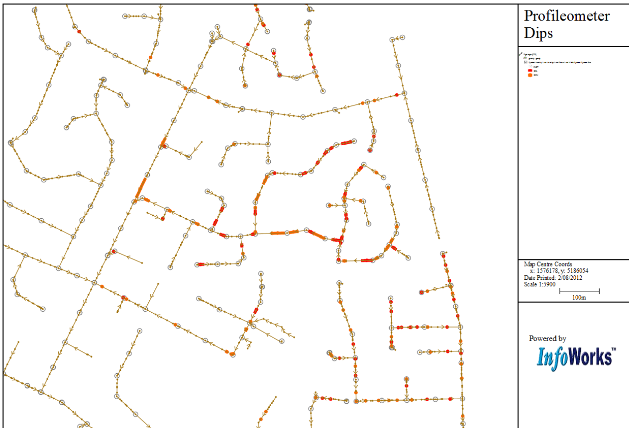
Figure 6: InfoNet plot of dips in WW network based on Profilometer Survey
