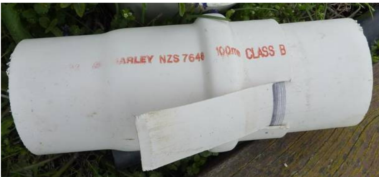
Figure 4: Re-insertion failure of PVC pipe
