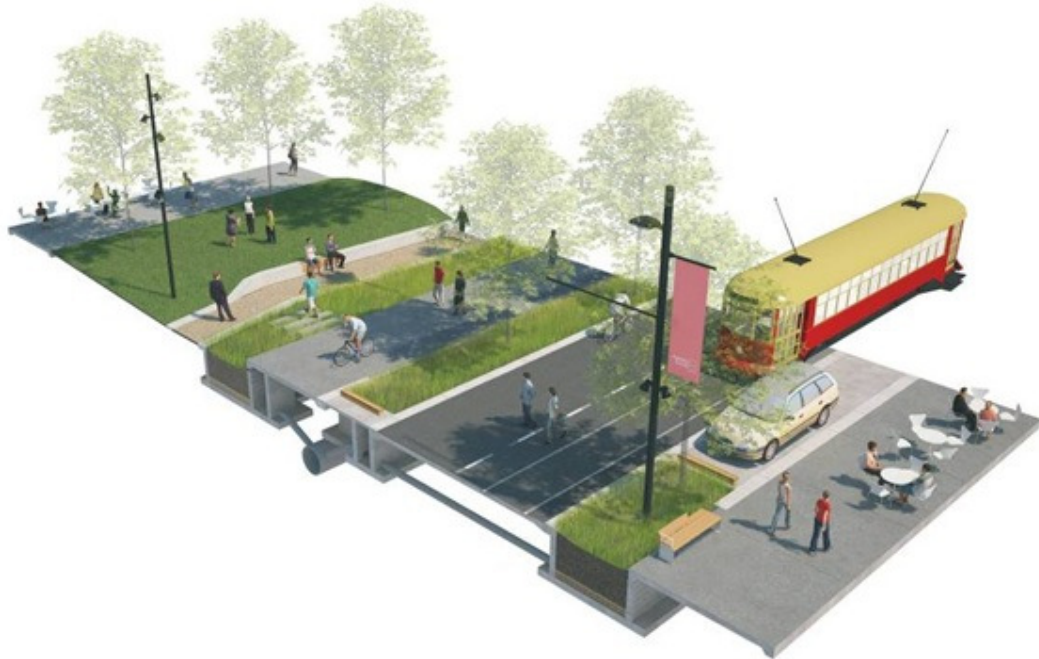
Figure 8: Overview of the Daldy Street Stormwater Management System
