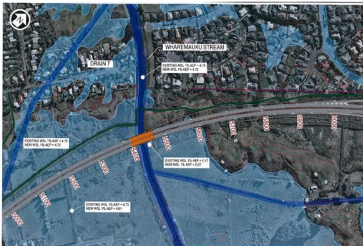
Figure 6: Part of an M2PP flood map prepared for the AEE showing the Wharemauku Stream, 1% AEP floodplain, proposed Expressway and a local road crossing the floodplain.
