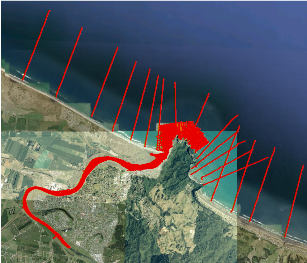
Figure 3: Discovery Marine Limited bathymetric survey coverage.
