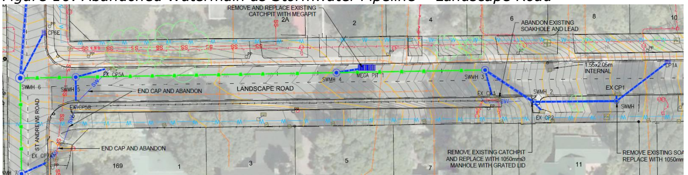
Figure 16: Abandoned Watermain as Stormwater Pipeline – Landscape Road
