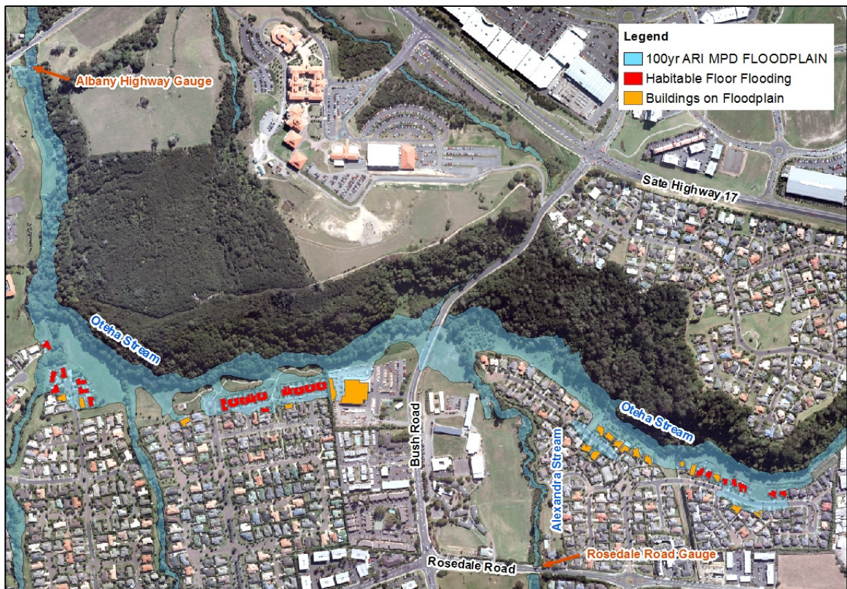
Figure 7: Oteha Stream 100yr ARI MPD floodplain with habitable floor flooding
