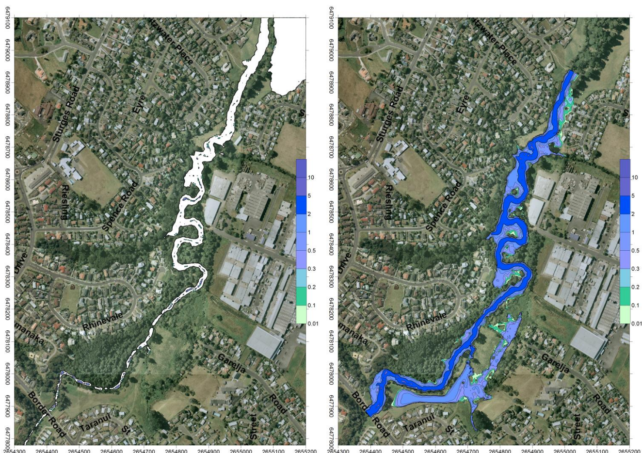
Figure 11. Flow Depth Contours of Verification Event at 0000 (Left) and 1300 (Right)
