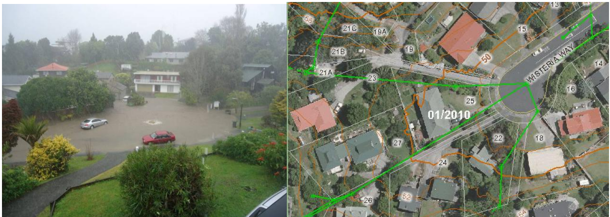
Figure 7 (A) A popped manhole in the middle of a flooded cul de sac; and (B) the incoming and outgoing pipes to and from this manhole
