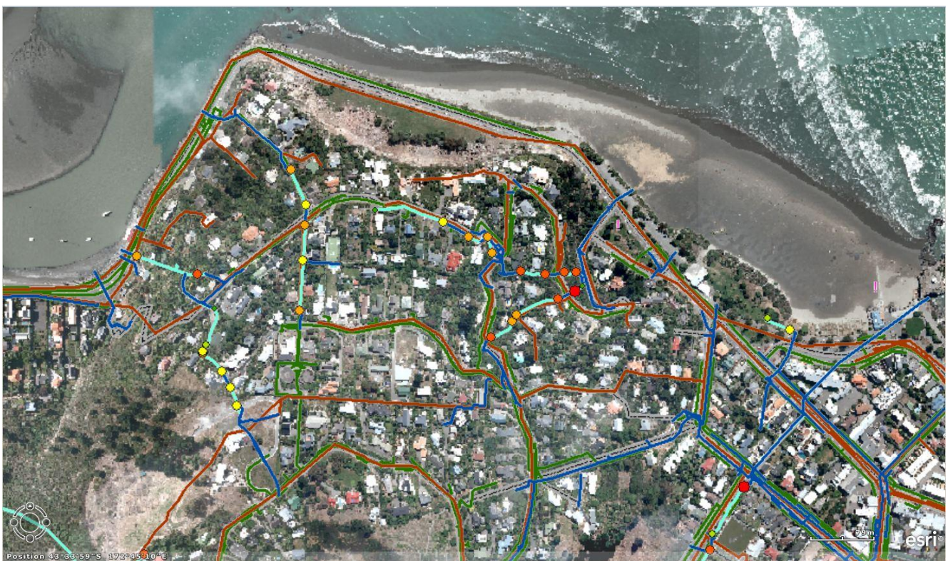
Figure 2: Example of the combined review data showing criticality score of each water course (coloured lines) and priority score colored dots. Refer to legend (below)
