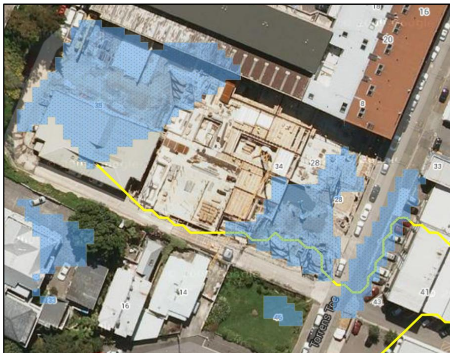
Figure 9: Overland flow path and depression area intersecting a site
