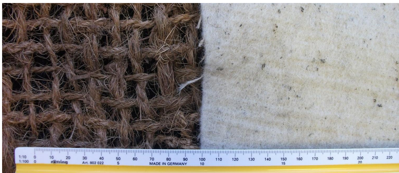
Photograph 1: 900\text{g/m}^2 coir fibre selected product (left) and the 450\text{g/m}^2 mixed coir fibre/wool substituted product (right).
