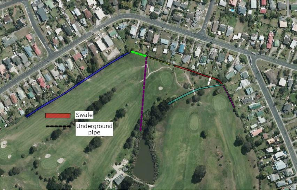
Figure 2: Swale network draining to Holding pond.
