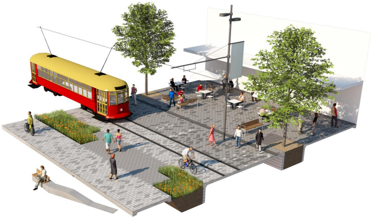
Figure 2 – A 3D rendering of the proposed urban landscape (Terraces) showing rain gardens on the left.
