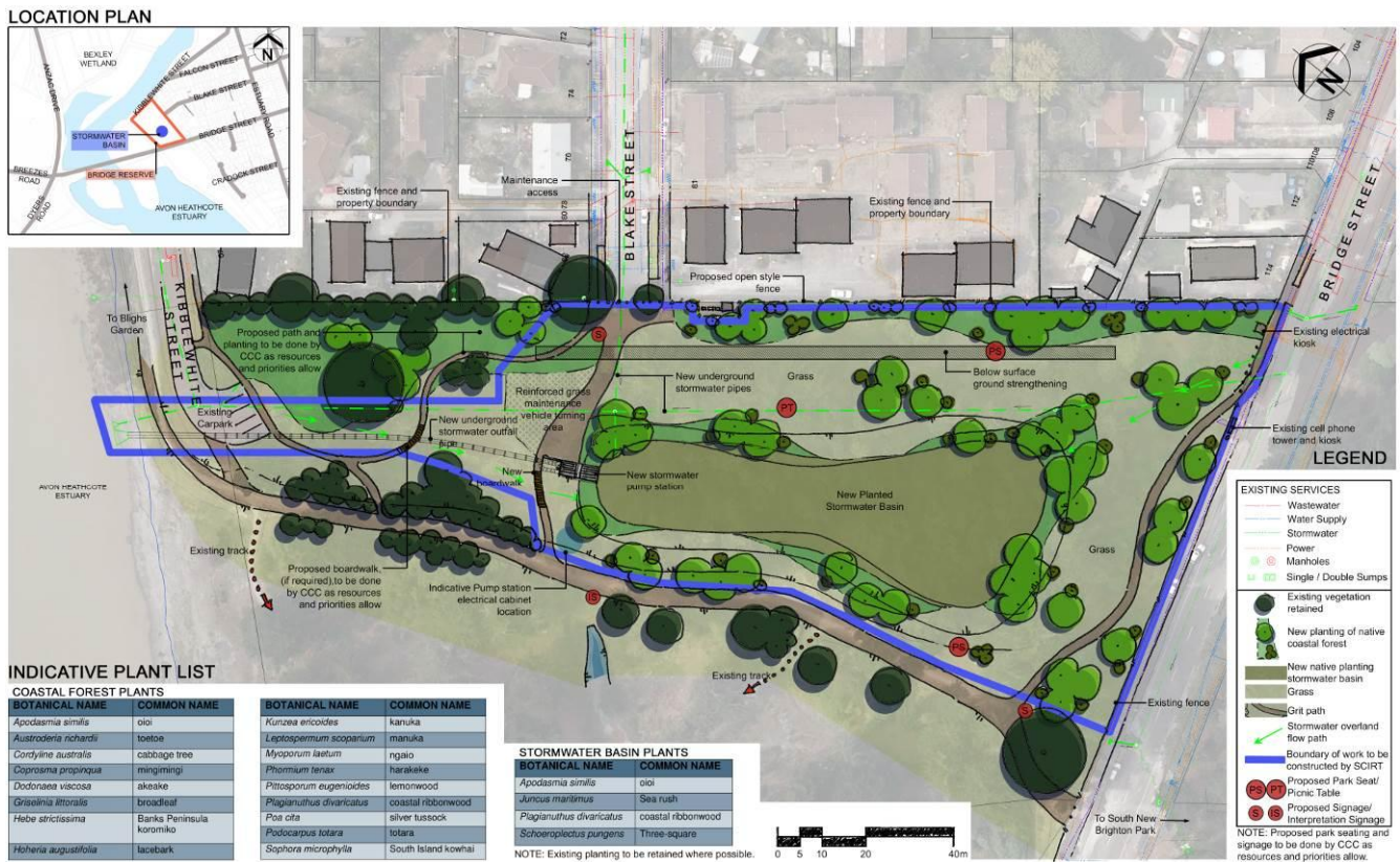
Figure 7: Final basin and pump station design layout
