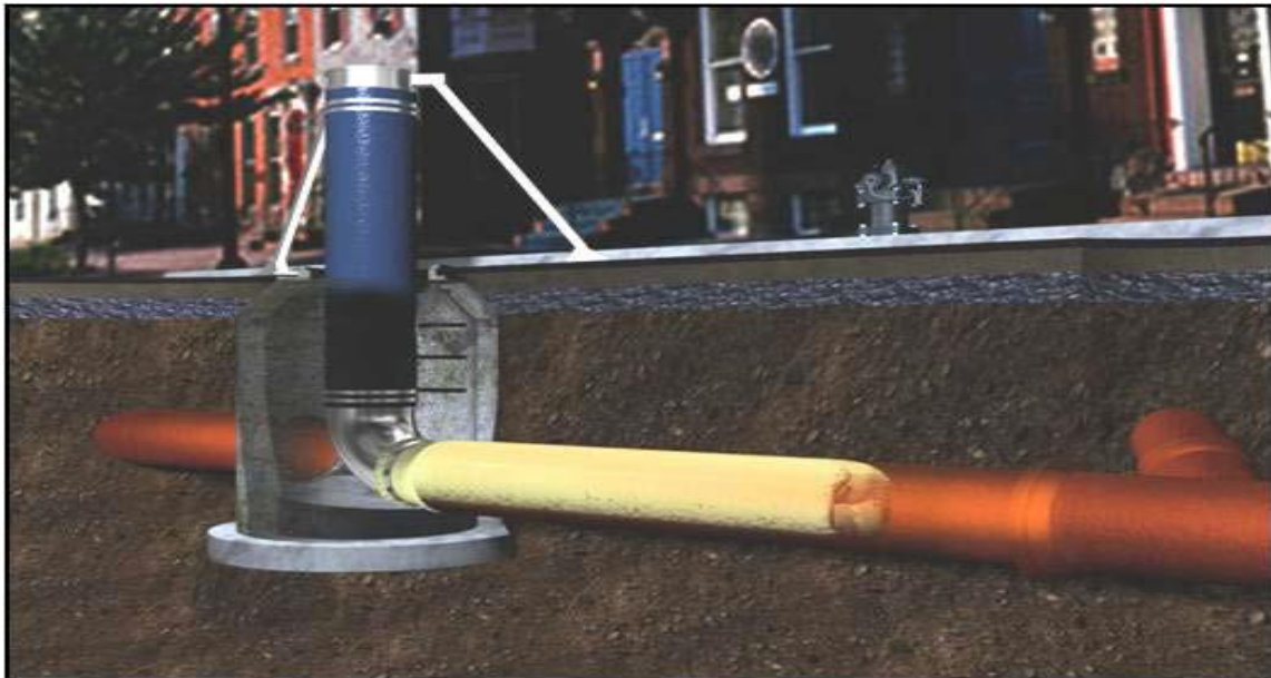
Fig. 15 CIPP Installation Liner Inversion - (Courtesy Insituform Technologies, Inc.)
