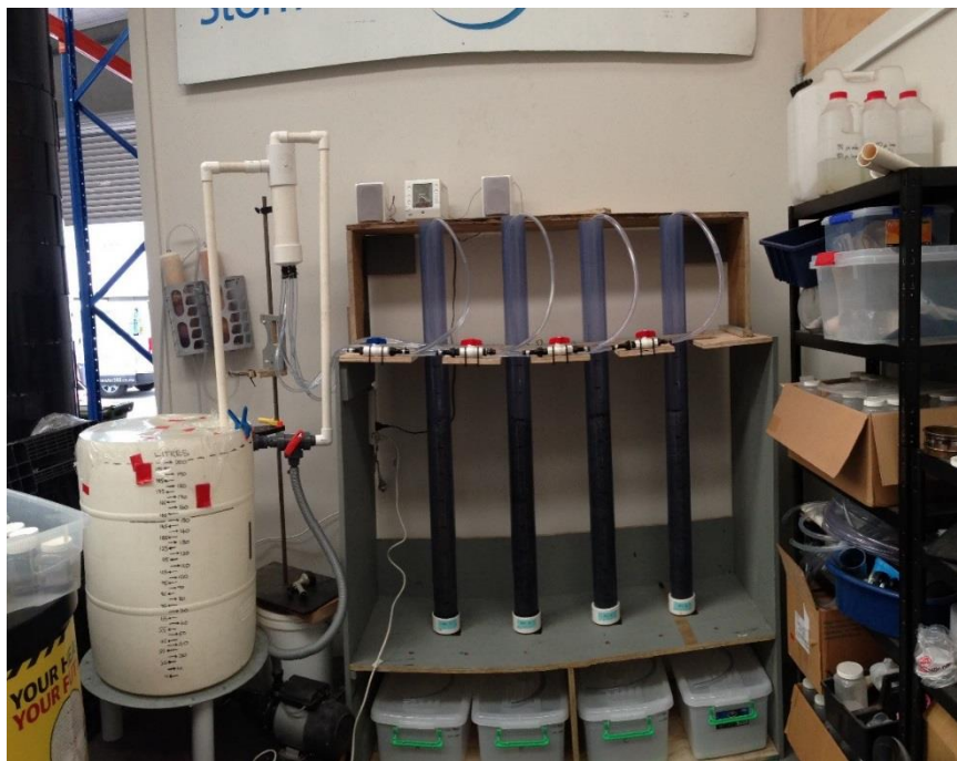
Photograph 2: Four column test setup at Stormwater360
