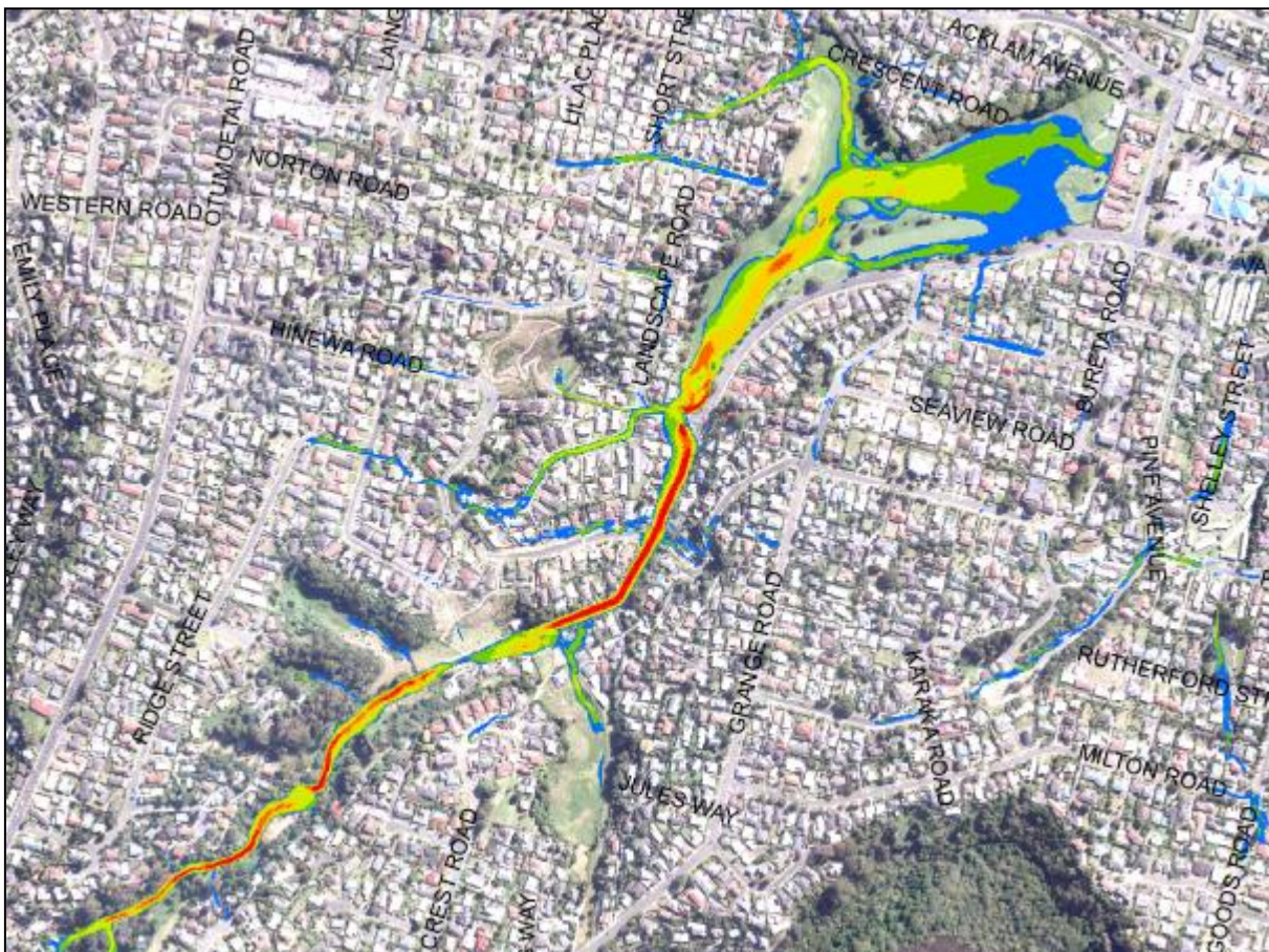
Figure 4: Example of Depth-Velocity Map – Pillans/Bureta Modelled Catchment.
