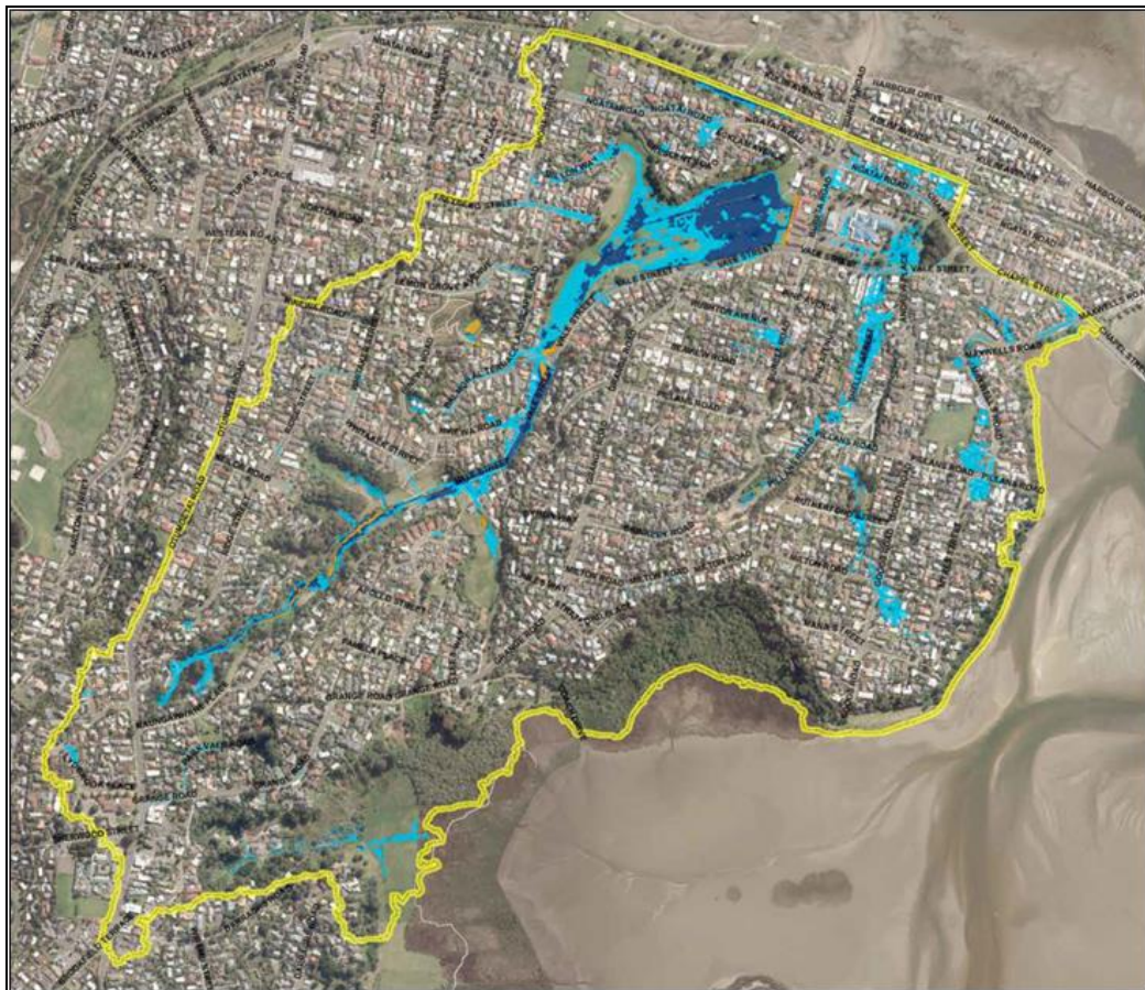
Figure 1: Flood Map (Depth) 100 year Existing Development – Pillans/Bureta Modelled Catchment.
