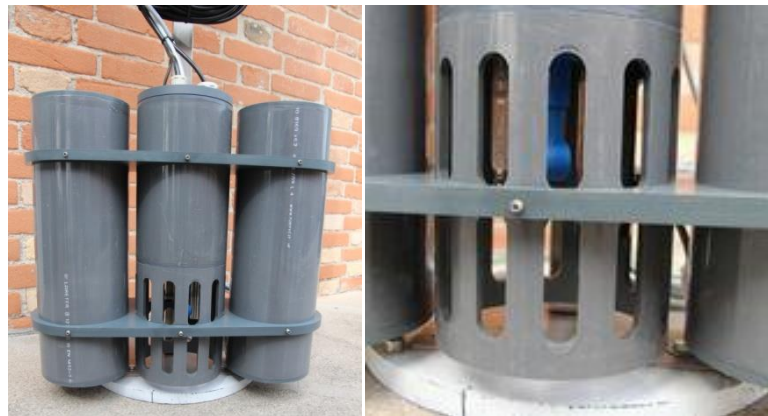
Figure 2: probes housing with a collision protection system
