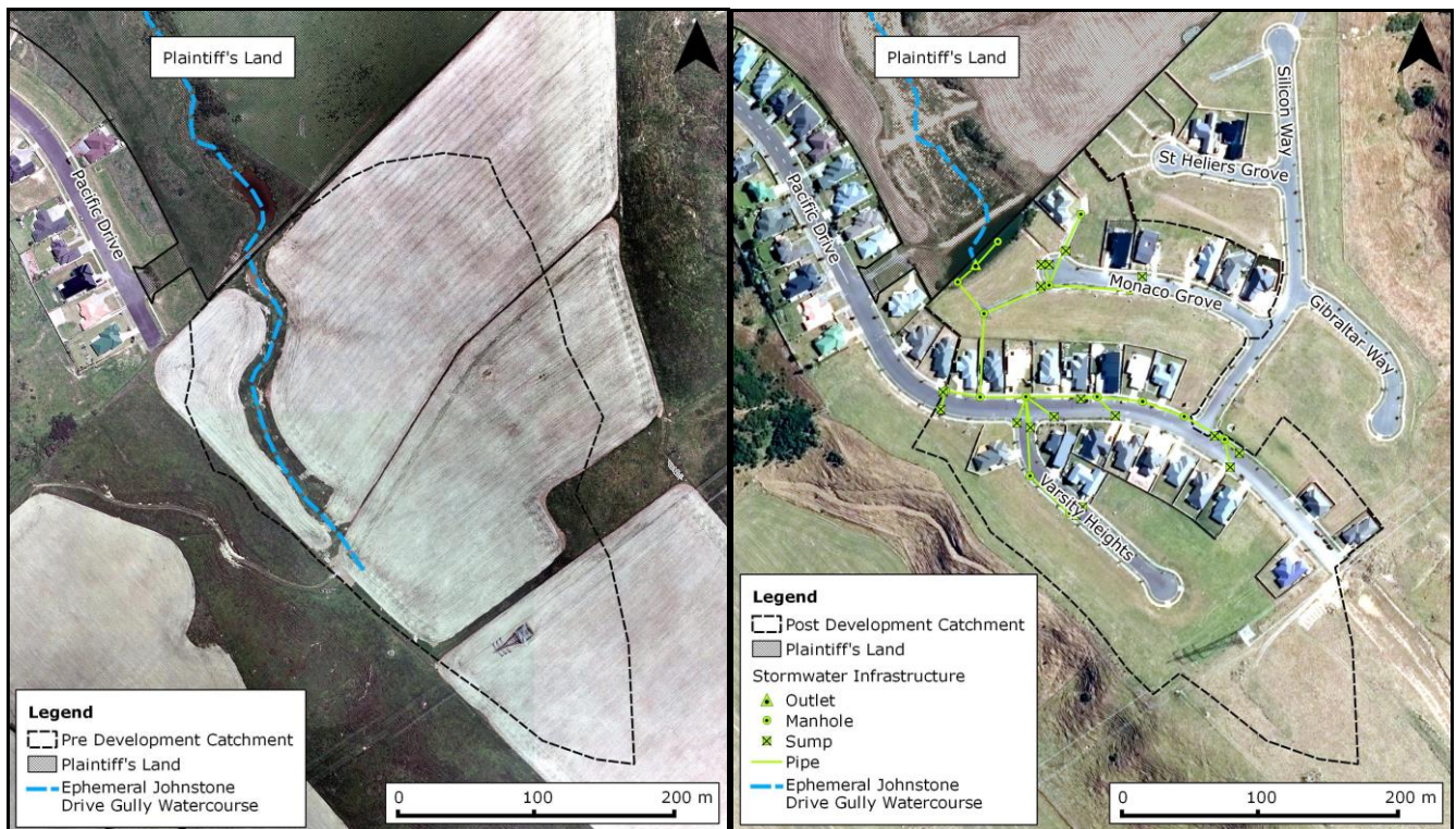
Figure 1: Johnstone Drive Gully Catchment Pre and Post the Development of the Pacific Heights Subdivision
