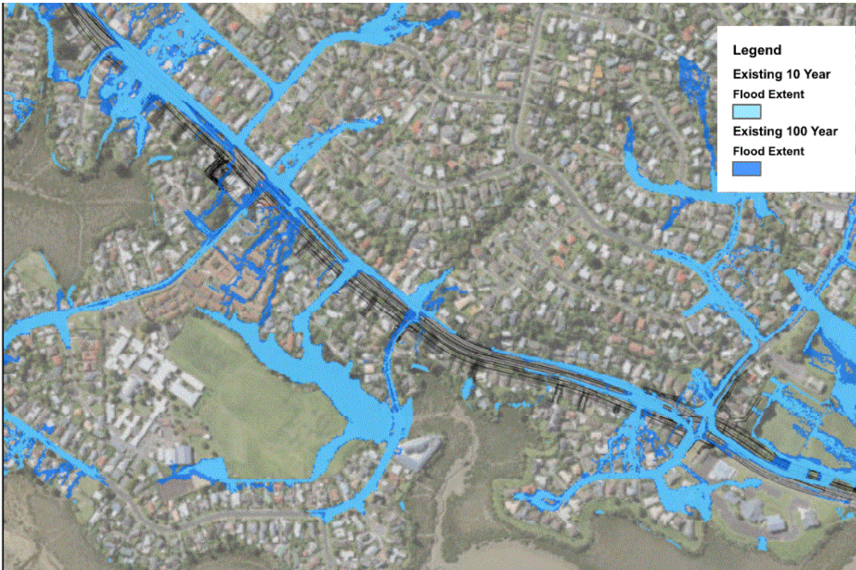
Figure 6: EB3R base case 10% and 1% AEP flood extents.
