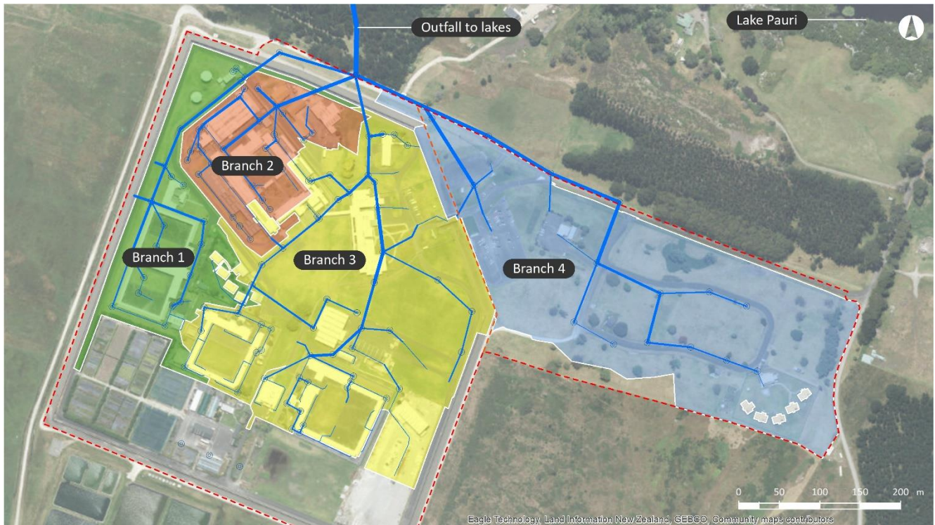
Figure 3. Prison catchments and piped stormwater network
