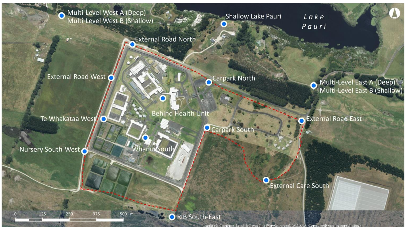
Figure 5. Piezometer network at Whanganui Prison Stormwater Conference & Expo 2024
