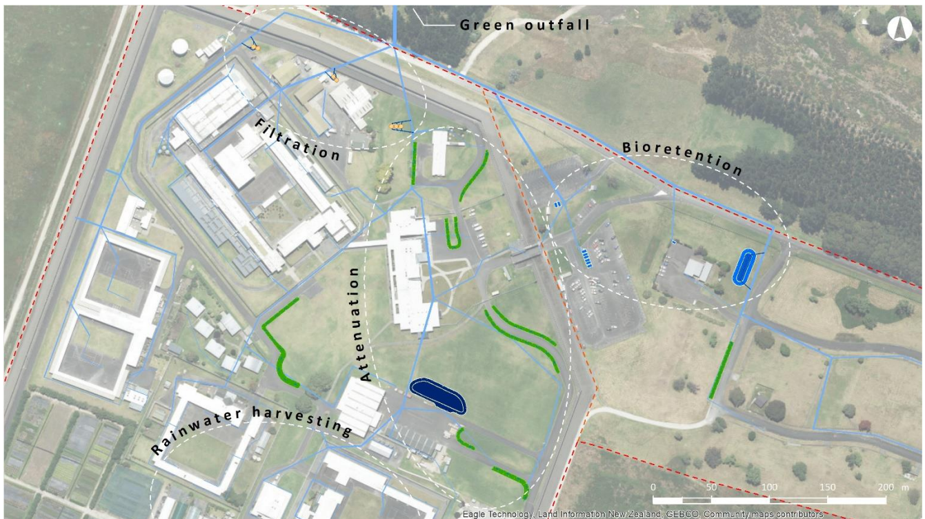
Figure 7. Layout of final treatment design
