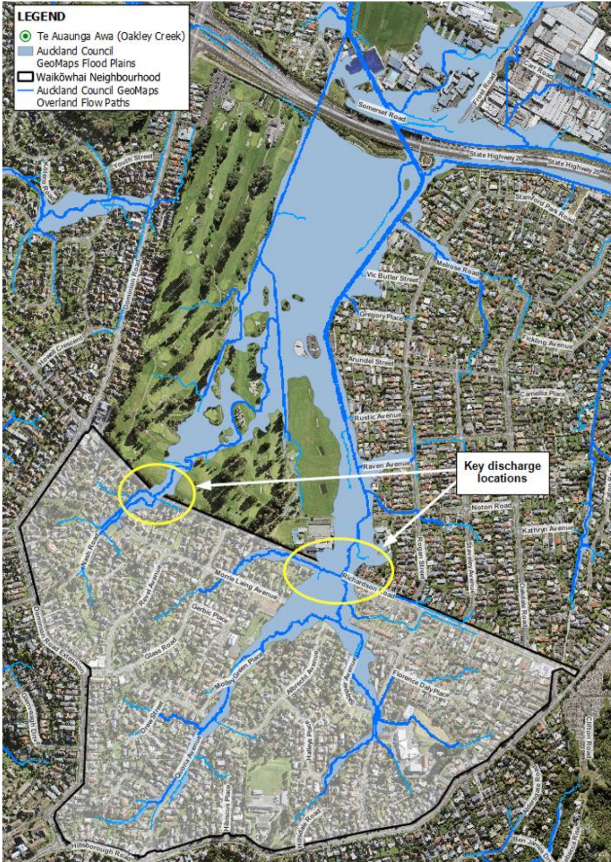
Figure 4: Two key discharge locations along low points at Richardson Road
