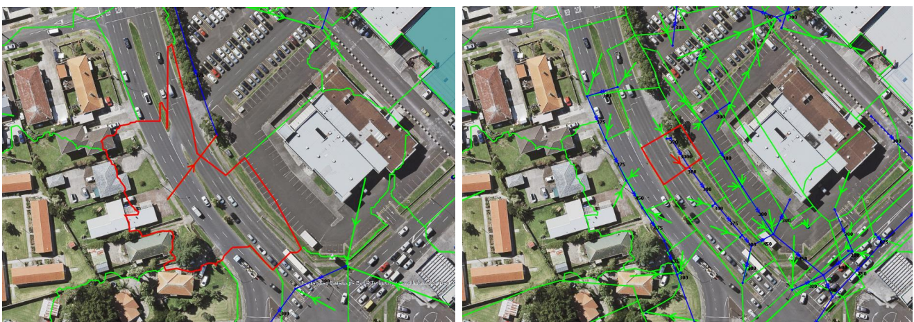
Figure 9: Comparison of a 0.3 ha subcatchment outlined in red in the Auckland Council flood model on the left with a 0.03 ha subcatchment in the EB2-EB3R flood model on the right.
