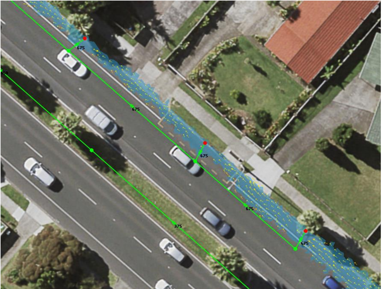
Figure 7: Example of the design model catchpits shown in red within the overland flow path and the manholes shown by the green nodes not within the overland flow path.
