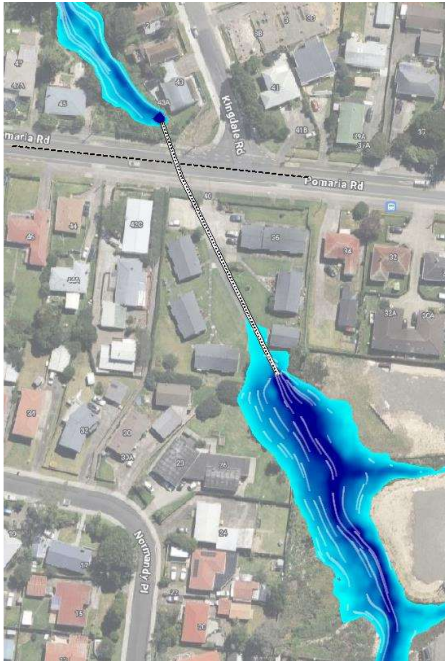
Figure 9: MPD CC culvert upgrade
