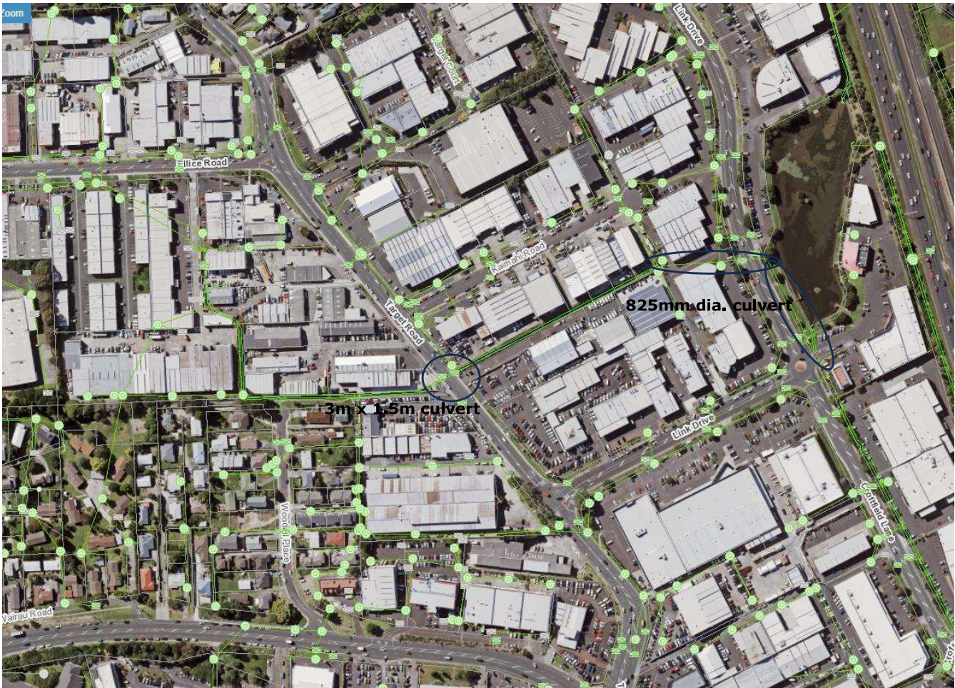
Figure 10: Target Road Culvert and Link Drive Culvert (Source: Auckland Council GeoMaps)
