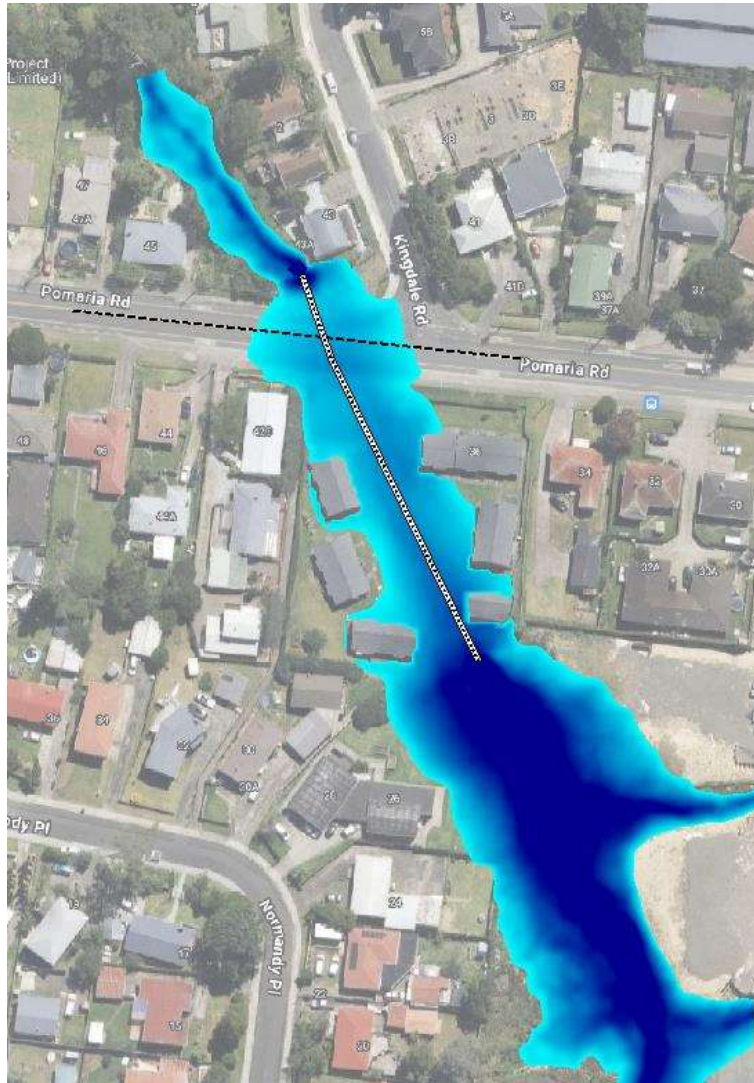
Figure 7: Existing Culvert MPD + CC
