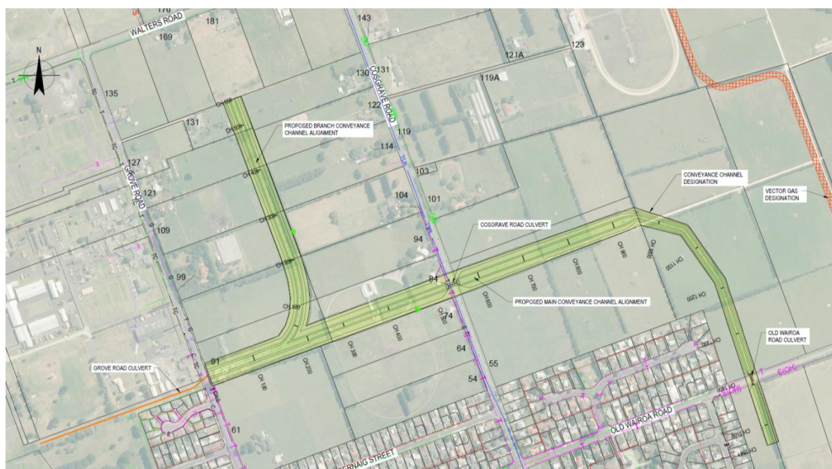
Figure 5: Proposed Takanini stormwater conveyance channel
