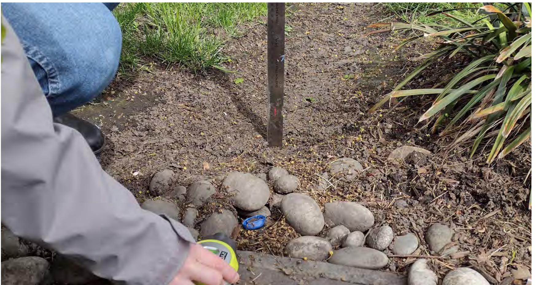
Measuring ponding depth near outlet with no vegetation blocking laser
