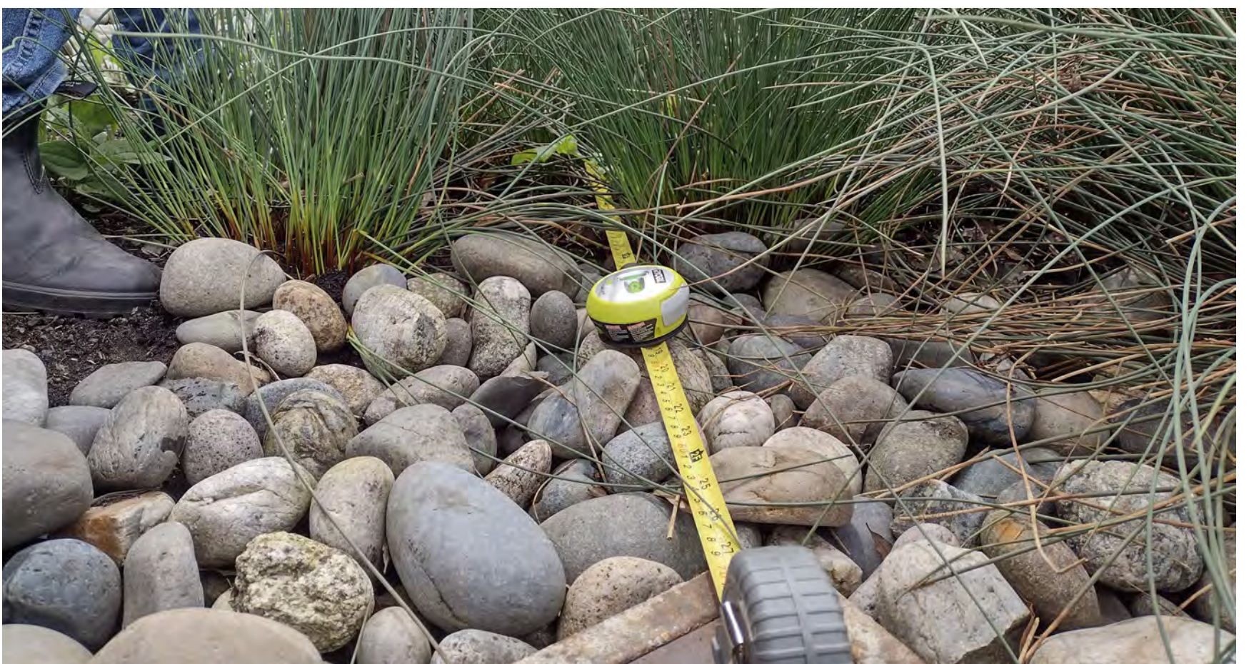
Measuring ponding depth when vegetation is blocking laser
