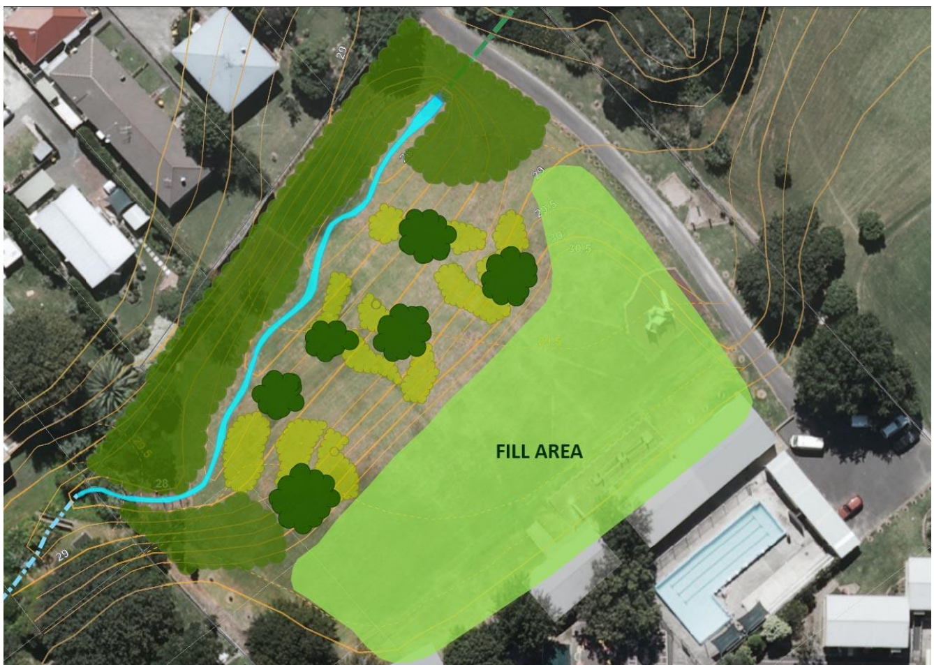
Figure 1: The concept plan showing the stream meander and the residual level field area which is to be raised 1.6 metres using material excavated to form the stream.
