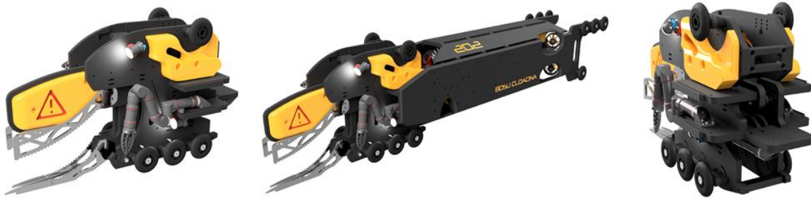
Figure 6: Renders of Debris Removal – Detached and Installed
