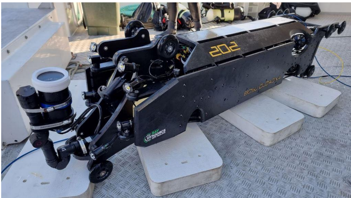
Photo 10: ROV with Inspection Payload
