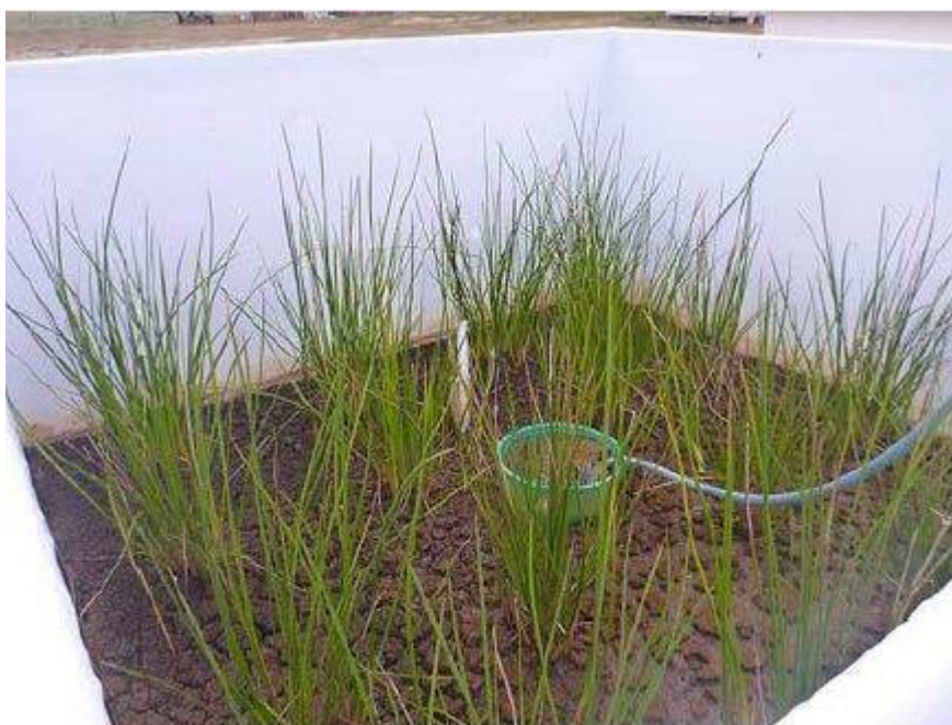
Photograph 7: Reed Bed Trial at Waikouaiti WTP
