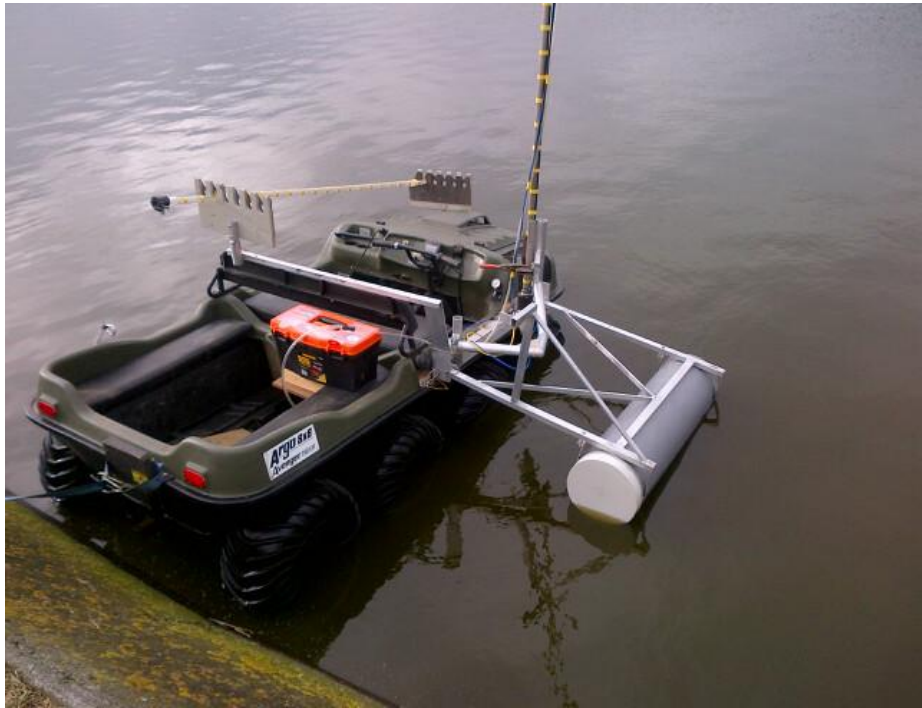
Photograph 3: Sampling rig showing version 2 vacuum sampler and sludge judge
