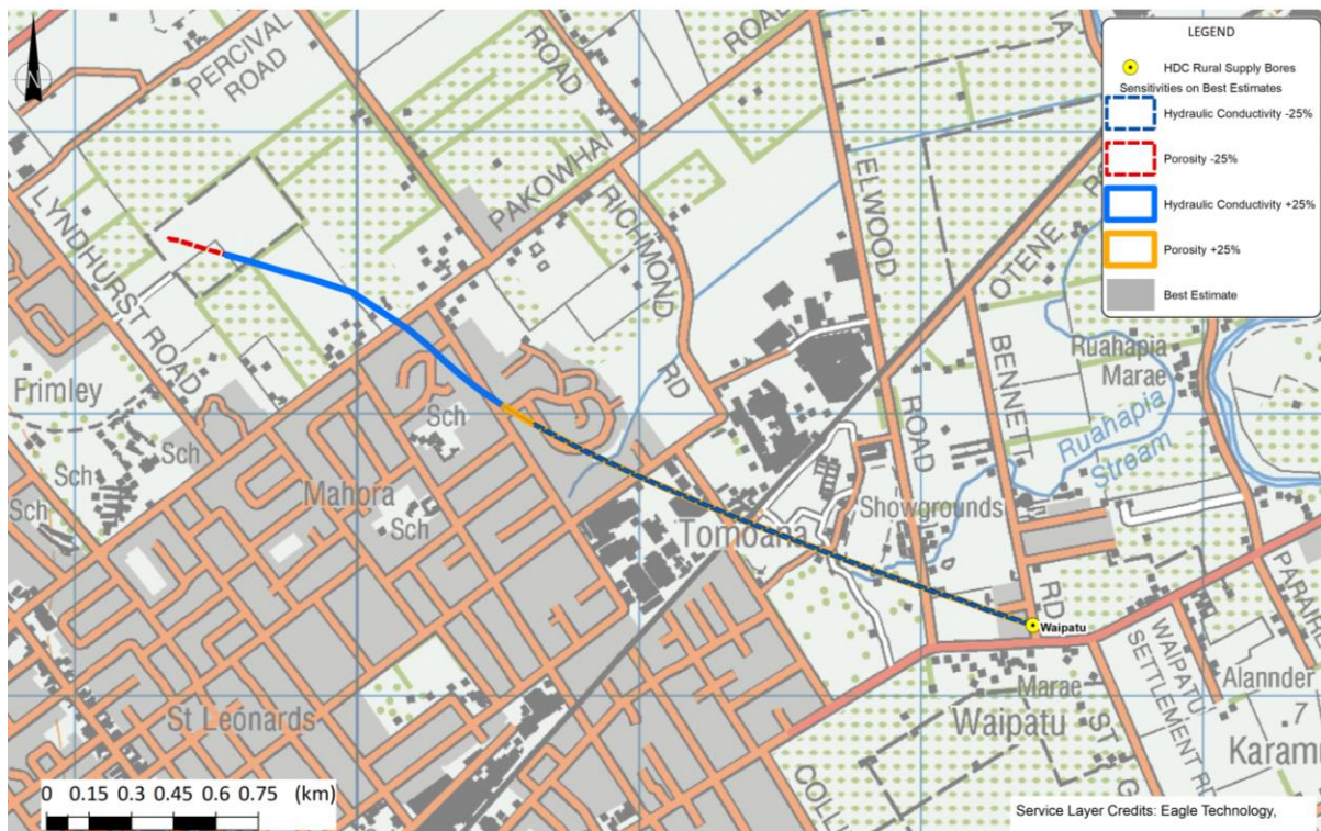
Figure 3a: SWRMA2 (SPZ2) for the Waipatu drinking water supply. Pathlines from the aquifer parameter sensitivity modelling runs for porosity and hydraulic conductivity.
