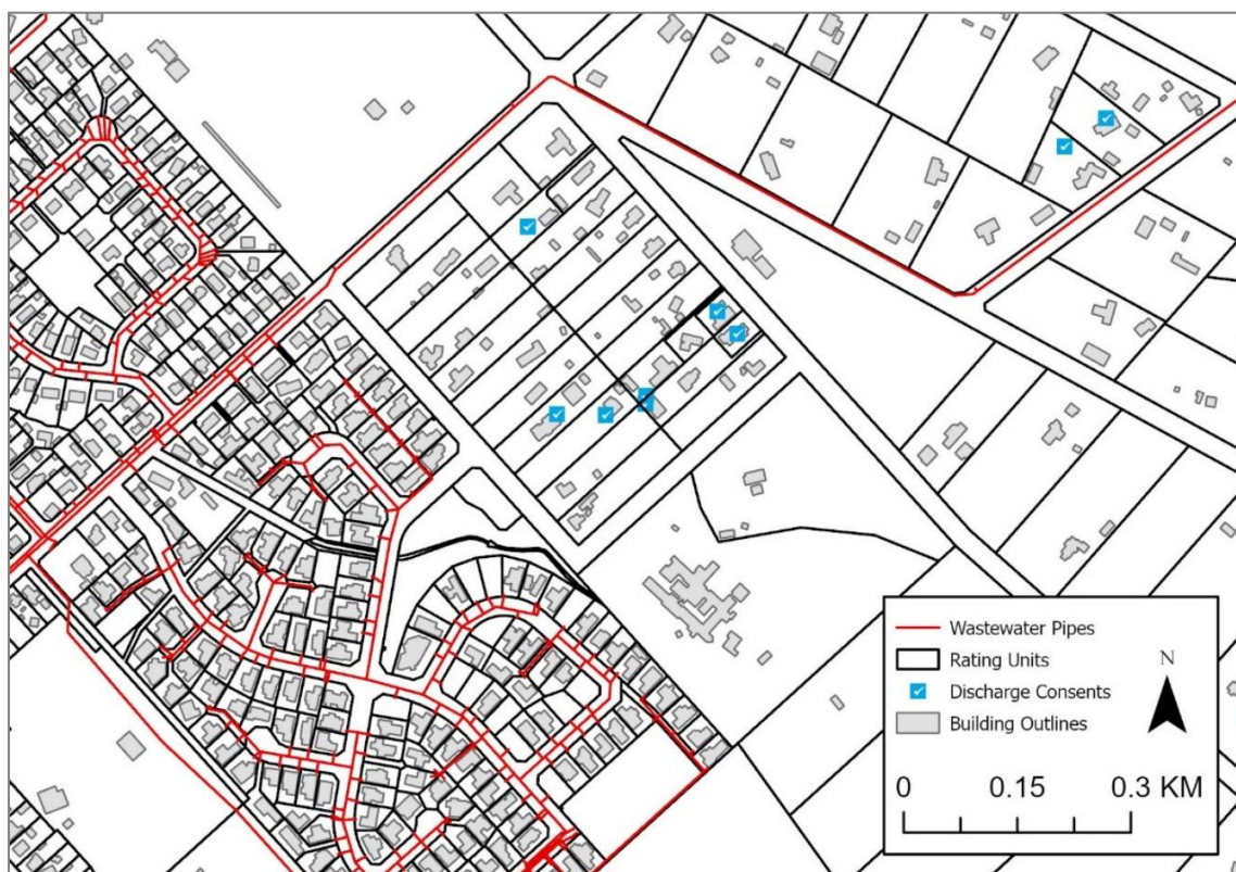
Figure 1: Map layers in Canterbury maps used in pinpointing unknown on-site wastewater systems (The map shows southeast of Ashburton town centre)
