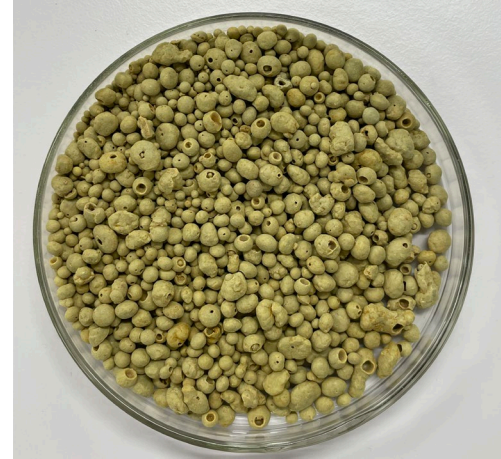
Sulfur composite ( S^0 + FeCO_3 ) granular packing media material
