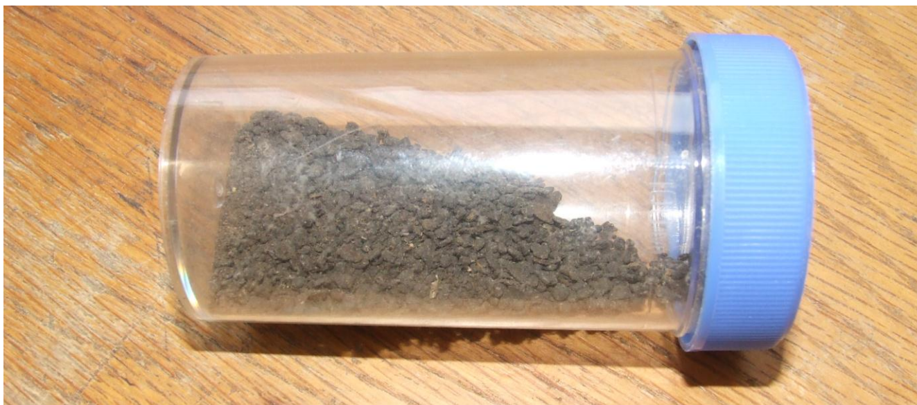
Photograph 5: A Sample of the Paraparaumu Dried Biosolids
