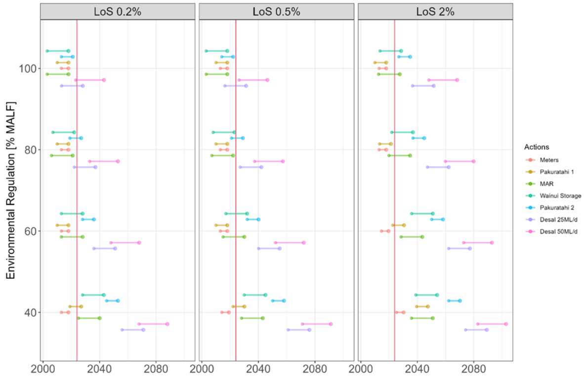
Figure 5: The influence of environmental regulation [MRF as % of MALF] and the Level of Service on the timing of the actions (when it has to be completed + the line shows the respective lead time).
