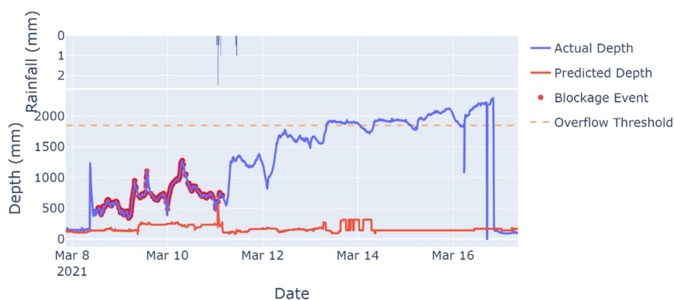
Figure 3: Positive Detection of Significant Blockage Event. Detection is shown in red. Successfully detected due to increase in actual depth (compared to predicted depth in red) outside of a rain event.
