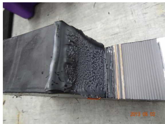
Photograph 11: Ductile Failure after testing
