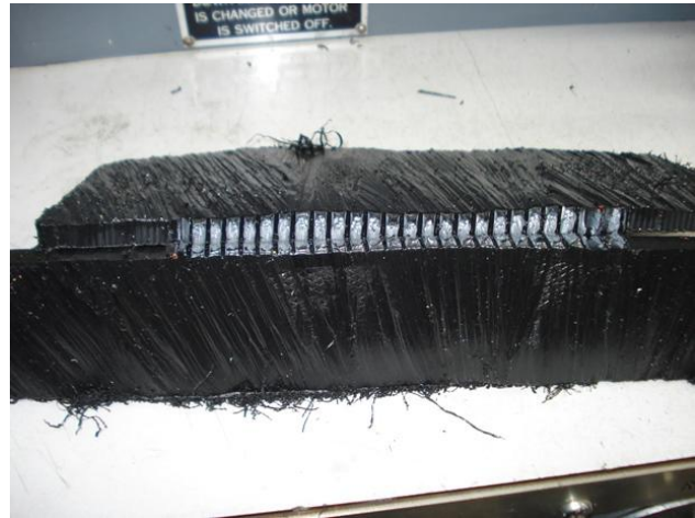
Photograph 13: Ductile Failure after testing
