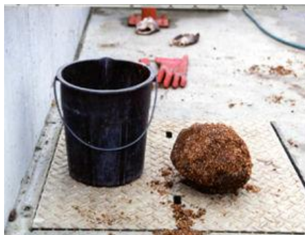
Figure 2: An example of mudballing – mudball found in a filter at Traralgon, Australia 2 .
