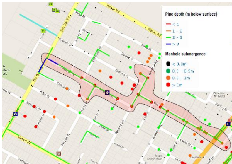
Figure 12: Network Submergence and Pipe Depth
